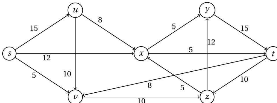
Run the Ford-Fulkerson algorithm to compute a max  $s - t$ -flow. For each iteration give the residual network and mark the path you choose for augmentation.
