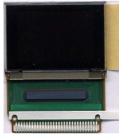
Fig. 3 Sample of a commercial OLED device with integrated driver chip
