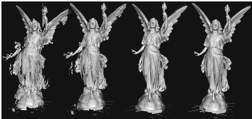
Figure 5.10: Alignments of the 368 patches of Lucy. Left to right: rotations are synchronized with EIG, LUD and MLE+. The fourth image depicts the reference alignment.
