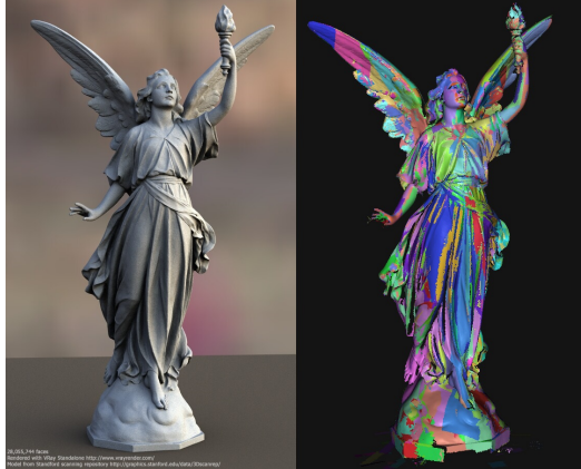
Figure 5.9: Left: virtual representation of Lucy provided by the Stanford 3D Scanning Repository. Right: representation of the subset of 368 scans of Lucy (each in a different color) with their reference alignment, using trimesh2.
